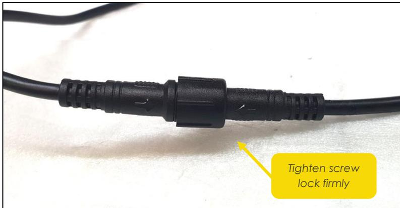
4. It is recommended to use a 40mm length of Ø14mm (minimum) heat shrink over each control plug to further act as a barrier to water ingress, as well as holding the screw lock in place over the life of the connection.
