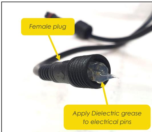
2. Align the arrows on the 2 mating plugs to ensure the keyways are positioned correctly. Firmly push the male plug into the female plug, noting that some Dielectric grease should flow out of the plug. Push firmly until the red O-ring is properly seated against the shoulder of the female plug and wipe away excess grease.
