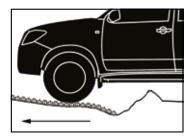
3. Using Low Range, slowly drive off in the direction that you have prepared and laid the X-Trax II. At all times, avoid wheel spin on X-Trax II.
