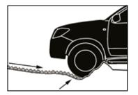
2. Place X-Trax II as far under that side of the wheel, against the tyre. Push the earth back under X-Trax II to ensure it is touching the tyre. Repeat for each bogged wheel.
