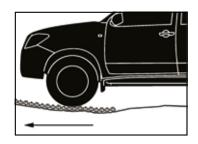
Using Low Range, slowly drive off in the direction that you have prepared and laid the X-Trax II. At all times, avoid wheel spin on X-Trax II.
