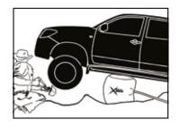
2. Pack as much earth as possible under wheel, lay down X-Trax II and place tyre on top of end furthest away from direction of travel. Repeat for each bogged wheel.
