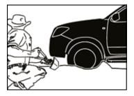
1. Use a shovel to clear enough area under wheel in the direction of recovery. Caution: Ensure vehicle is stable.
