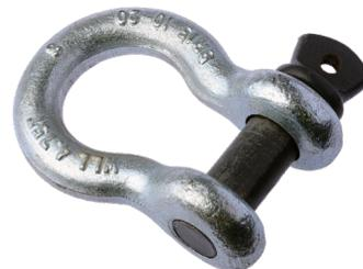
Never over-tighten the shackle pin. Forces exerted on the shackle by vehicle recovery can cause the pin to seize. The correct method is to tighten the pin until it seats, then back off the pin approximately 1/2 to 1 full turn.
