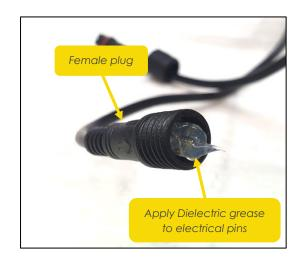
1. Apply a liberal amount of di-electric grease to the 4 pins of the control plug.
