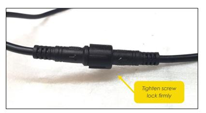
4. It is recommended to use a 40mm length of Ø14mm (minimum) heat shrink over each control plug to further act as a barrier to water ingress, as well as holding the screw lock in place over the life of the connection.
