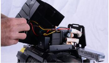
3. Remove the screws that hold the control plug wires to the contactor and detach these current control plug wires.
