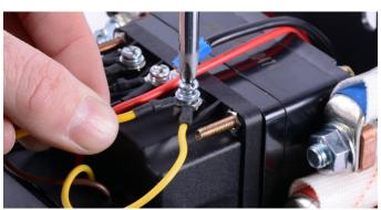
8. Replace the control box cover and fit the 4 original screws.
