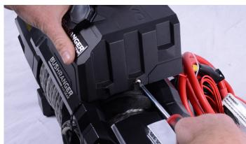
2. Lift the cover to reveal the coloured control plug wires.
