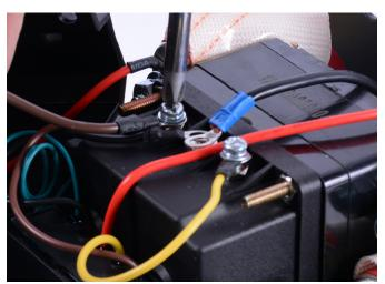
4. Undo the 13mm bolt and nut slightly to release the red wire.
