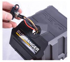
6. Install the new extended control box plug by feeding the wires through the hole in the control box cover where the original control plug was removed.
