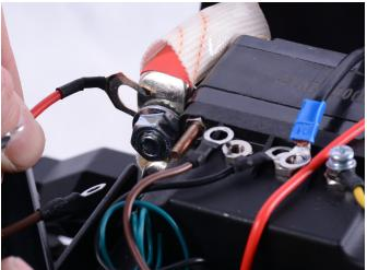
5. Undo the backing nut on the control plug and discard plug assembly.
