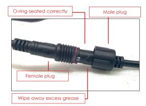
3. Tighten the screw lock to form a secure, waterproof connection. Ensure metal to metal contact between the electrical pins has been retained by trialling the full operation of the Variable Series wiring system before finalising the installation.
