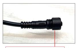
Fill plug with di-electric grease, then fit suppllied cap
