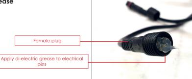
2. Align the arrows on the 2 mating plugs to ensure the keyways are positioned correctly. Firmly push the male plug into the female plug, noting that some Dielectric grease should flow out of the plug. Push firmly until the red O-ring is properly seated against the shoulder of the female plug and wipe away excess grease.
